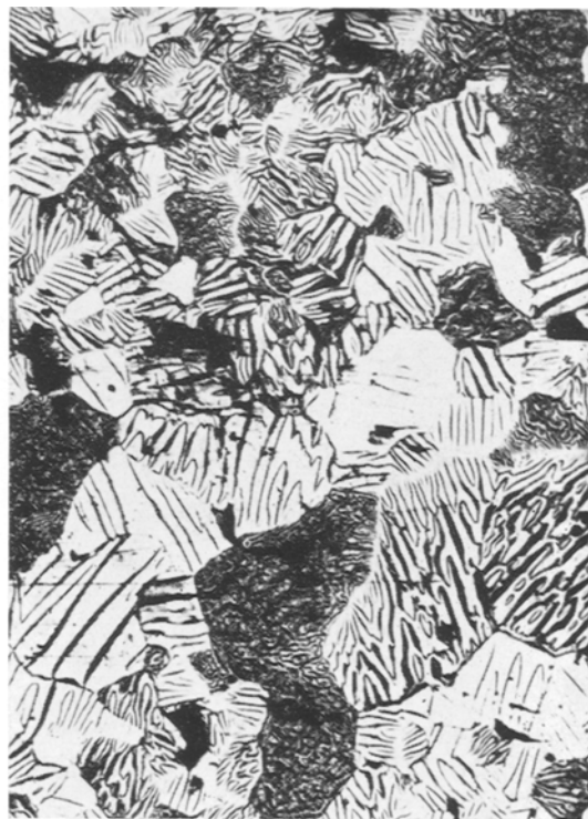
Figure 7 Domain structure on cast \text{CeCo}_5 ( \times 170 ). Coercivity < 200 Oe.
