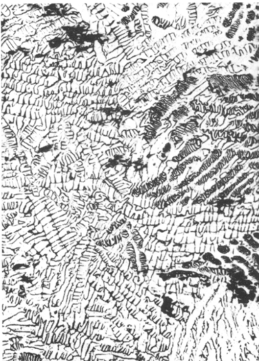
Figure 3 Domain structure on annealed SmCo 5 ( \times 170 ). Coercivity 550 Oe.
