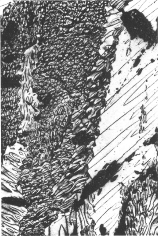
Figure 2 Domain structure on cast SmCo 5 ( \times 133 ). Coercivity 550 Oe.
